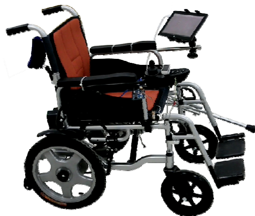
Figure 13. Electric Wheelchair with Hand-Gesture Intelligent Control Module
