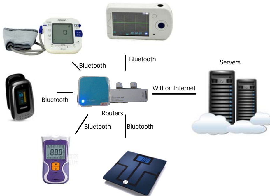
Figure 20. The Medical Devices for Aging Health Record Measurement and Collection
